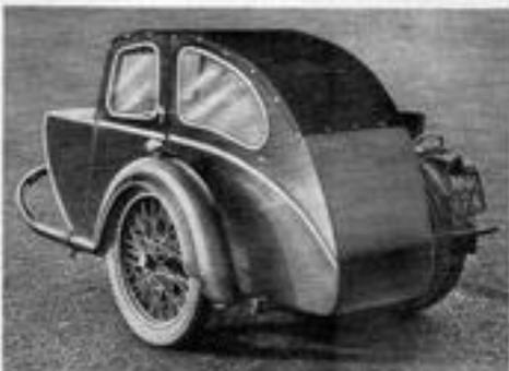
The saloon has a good streamline contour, which materially assists high-speed driving. Access to the rear locker is from inside the body.
